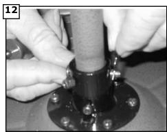
Insert cotter pin in to cross pin to secure.
